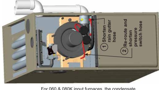
For 060 & 080K input furnaces, the condensate drain is plumbed toward the right casing outlet from the factory.
